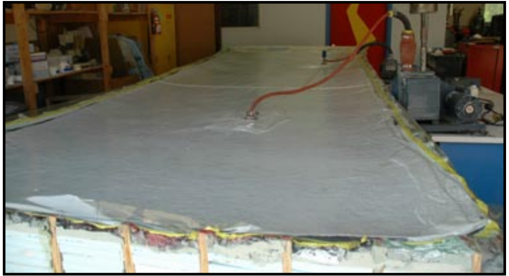
The new lower body rests in the mold, still sealed in the vacuum bag the morning after it was laid up.
