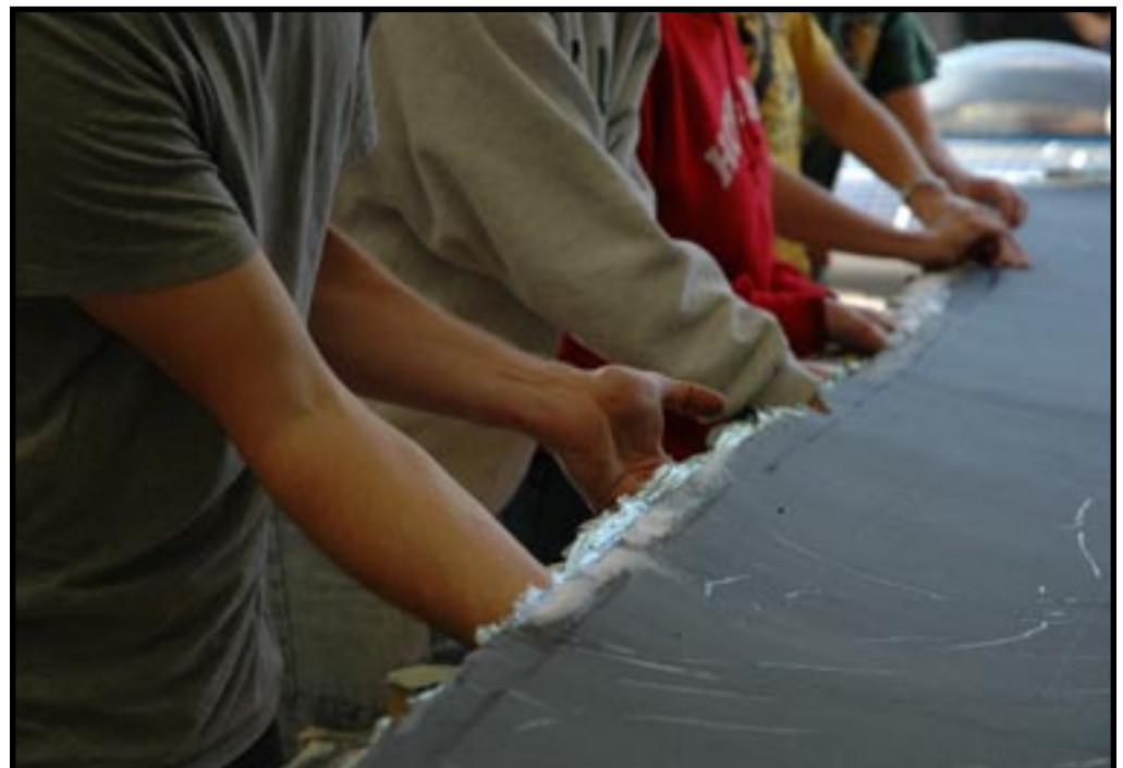
Team members remove the finished lay-up, the car's new lower body, from the mold to examine it.
