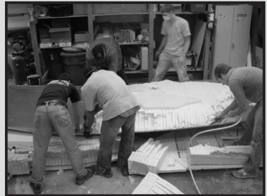
Top: Ribbing the new mold in order to provide structure.
