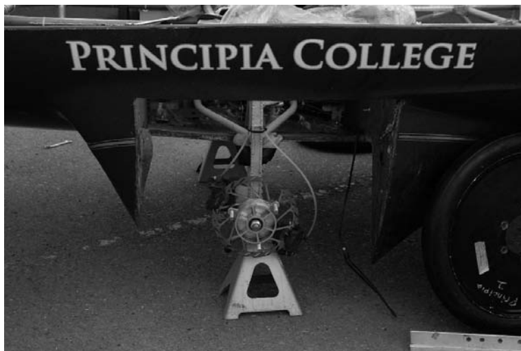
The mechanics behind the wheel: The hub mounts to the kingpin, and the brake rotor and caliper mount to the hub.
