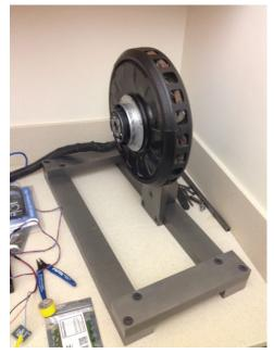
tor is that the magnets and coils lie in concentric circles as opposed to parallel to each other. The disadvantage of this is that it leaves less room to alter the distance between the coils and the magnets based on the voltage supplied to the motor. The way Mitsuba remedies this detail is by having teams provide the voltage of their car and Mitsuba custom designs the motor with the proper air gap.
