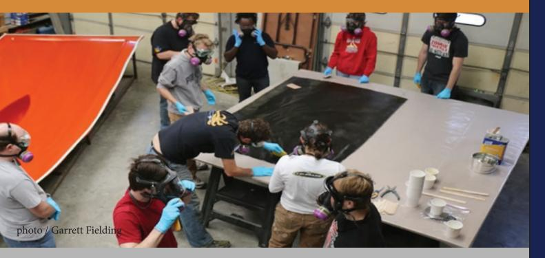
With the construction of Ra 10 in mind, we spent a Saturday in early November teaching students how to work with carbon fiber. The main body and structure of a solar car is comprised of carbon fiber, a flexible woven fabric that, once a hardening epoxy is added, can be molded to any shape, and becomes rigid, light and strong. Because carbon fiber is such an important material for the production of a new solar car, we need students with hands-on experience prior to the construction of Ra 10.
