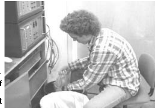
Eric Silver works his way through cycling 27 lithium ion modules in an effort to match them when wiring the pack.
