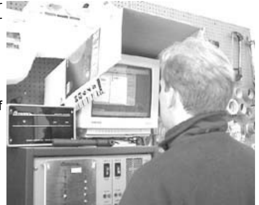
Nate Dudley sets up the Bitrode battery cycler, in an effort to test our new batteries.
