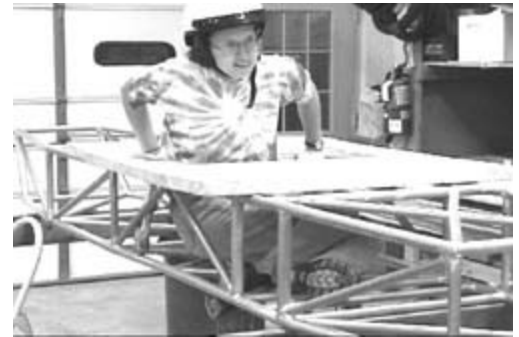
Allison Wiegand simulates the egress test in an effort to size the driver opening in the body.
