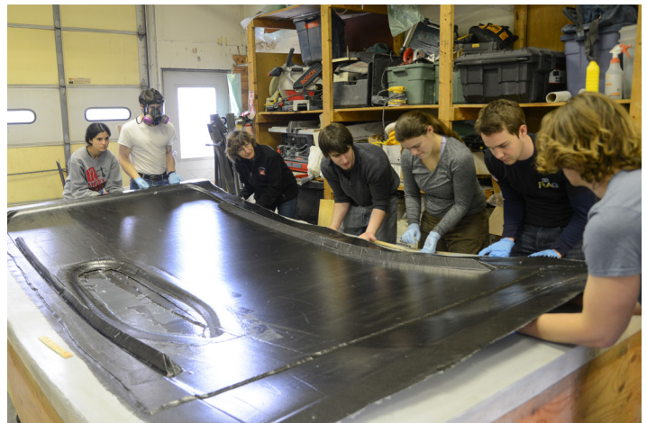
The team removes the upper body from the mold for the first time
