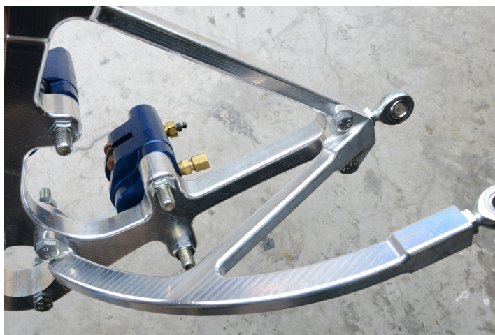
This milled aluminum trailing arm is lighter than a steel version
