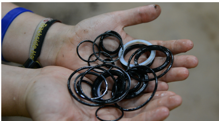
O-rings replaced from one of the air shocks
